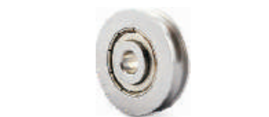
KT1602029 Model: Non-standard S5201-2RS Material: Stainless Steel SUS420 Size: 12*41*16mm
