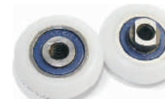
KT1600581 Mode:6001ZZ Steel Type: Stainless Steel/ GCr15 Chrome Steel Plastic Coat: POM/Nylon Size:12x47 × 16.3mm
