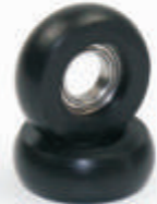
KT1601559 Model: 626ZZ Steel Type: Stainless Steel/ GCr15 Chrome Steel Plastic Coat: POM/Nylon Size: 6x30x6mm
